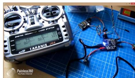
Be aware though that due to the inverted nature of the telemetry signals for FrSky receiver an inverter may be needed.
