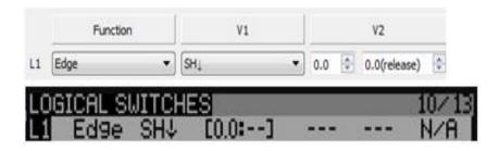
Using SH↓ as V1 and 0.0 and 1.0 as V2: the logical switch would be true as soon as SH was pressed down and released WITHIN 1 second. If it were held for longer than 1 second, this would not become true
