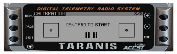
You should already know what this screen does. If you don't, then you didn't complete the **Checking Out Taranis** course and your transmitter is not calibrated. Performing calibration is necessary so that the Taranis knows exactly where the center and limits of each gimbal, pot, and slider is.
