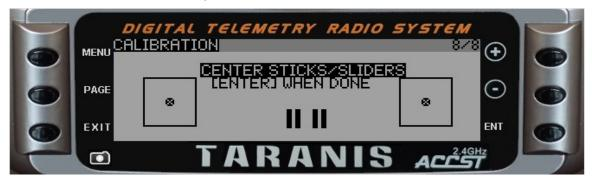
Now center both sliders, both pots. Now move the throttle stick to the CENTER of it's range, and make sure the other sticks are centered as well. Then press **ENT**, and you are done. The Taranis is now calibrated.
